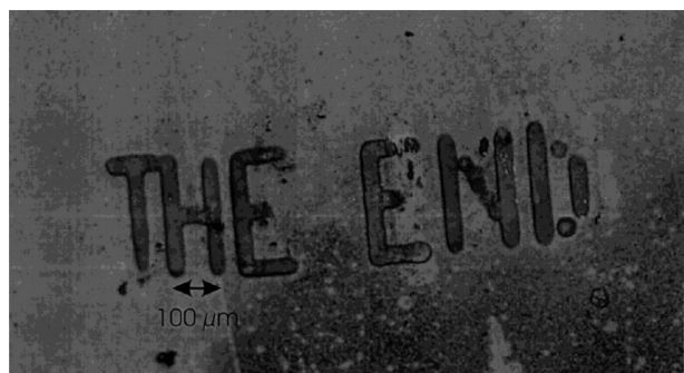
Figure 54. Micropattern of polythiophene obtained by local electrodeposition via SECM. Tip: 10 \mu\text{m} Pt, RG (shielding ratio) = 10, electrolyte = 40 mM \text{KNO}_3 , 20 mM thiophene, 10 mM \text{NaHCO}_3 . Galvanostatic process = 20 nA; scan rate = 0.8 \mu\text{m}\cdot\text{s}^{-1} at a distance of 8 \mu\text{m} from the surface; pattern width = 20 \mu\text{m} . Reprinted with permission from ref 502. Copyright 2001 American Chemical Society.
